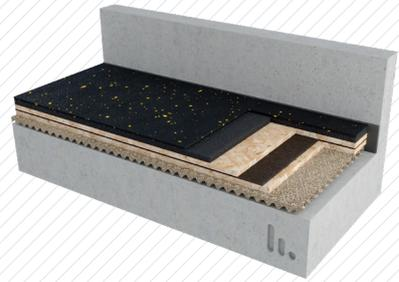
**!** If the Stravigym floating floor system is a different height to the surrounding structure an edge profile will be required. If a rigid edge profile is used ensure that the height of it is less than the height of the total floor system so that it does not make contact with the supporting floor after deflection of the system (**1** > deflection + creep).
