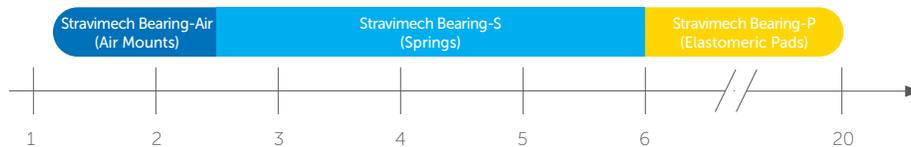
Figure 3 - Mount selection based on natural frequency ( $f_r$ ).
