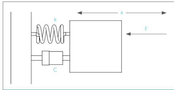
Figure 2 - Mass-spring-damper setup.
