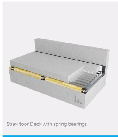
Stravifloor Deck is a [low-profile floating floor system](#) using a proprietary dovetailed metal deck for thin concrete pours. The system's high bending stiffness allows for concrete toppings as thin as 50 mm, making this system a great solution for projects that require a low-profile or lightweight concrete floating floor. It is also suitable for areas with high live loads.
