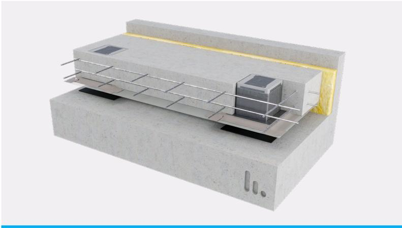
Stravifloor Jackup-R is an isolated floating floor system using [reinforced steel boxes](#) cast into concrete and jacked up after the concrete has cured, to provide the required void depth.
